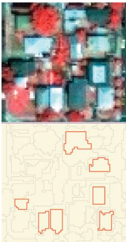
Figure 10. Building-oriented segmentation of the test building image subset ( 75 \times 70 ) by applying the suggested optimal parameter used in figure 9 (left). Available in colour online.
