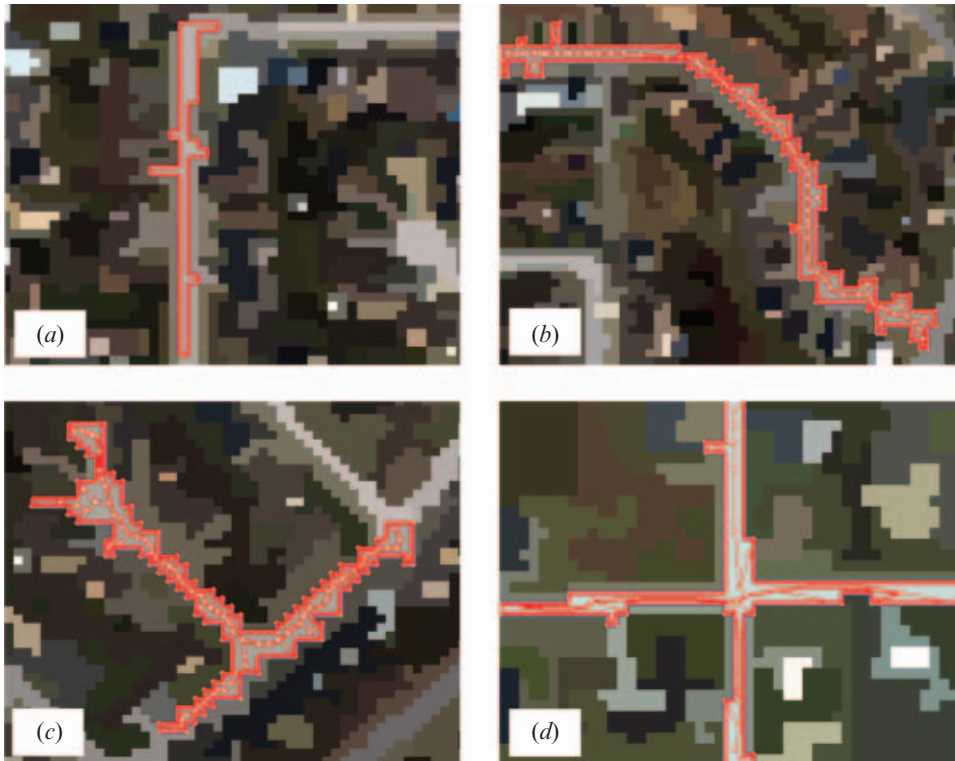
Figure 2. Four typical shapes of road objects. The upper two represent typical objects of connection; the lower two represent typical objects of intersection. The thicker inner lines represent the main lines. Available in colour online.
