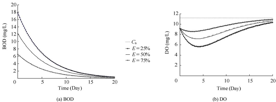
Fig. 1 Stream BOD and DO dynamics under different waste discharge scenarios from the plant ( $C_s$ : saturation DO at the average temperature of 10 °C)
