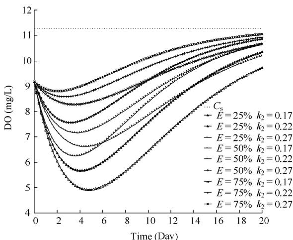
Fig. 4 DO sensitivity to the reaeration parameter ( $k_2=0.22/day$ ) based on boundaries of [0.17, 0.27] (mg/day)
