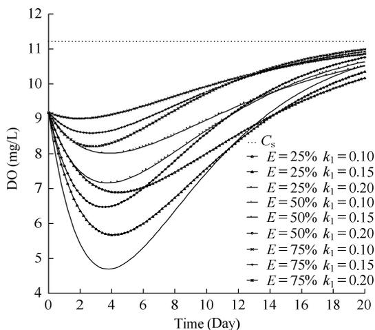
Fig. 3 DO sensitivity to the biological removal parameter ( $k_1=0.15/day$ ) based on boundaries of [0.10, 0.20] (mg/day)
