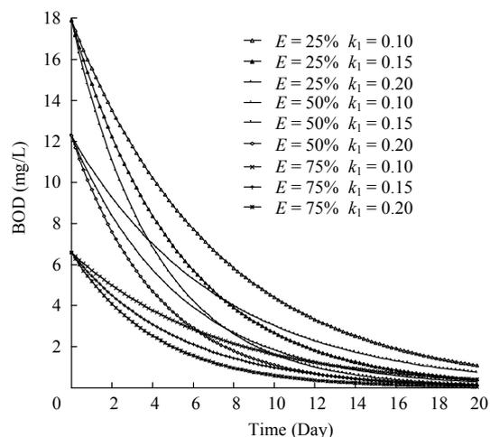
Fig. 2 BOD sensitivity to biological removal parameter ( $k_1=0.15/day$ ) based on boundaries of [0.10, 0.20] (mg/day)
