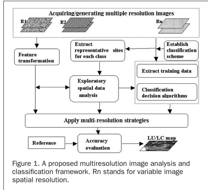
Figure 1. A proposed multiresolution image analysis and classification framework.  $R_n$  stands for variable image spatial resolution.
